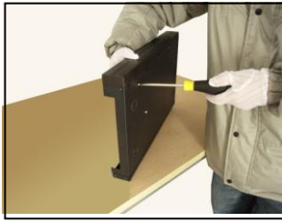
④fix the screw of hard disk
